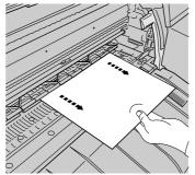
4 If the jammed sheet is not visible, on the back of the printer open the roll media guide then pull out the jammed sheet.
